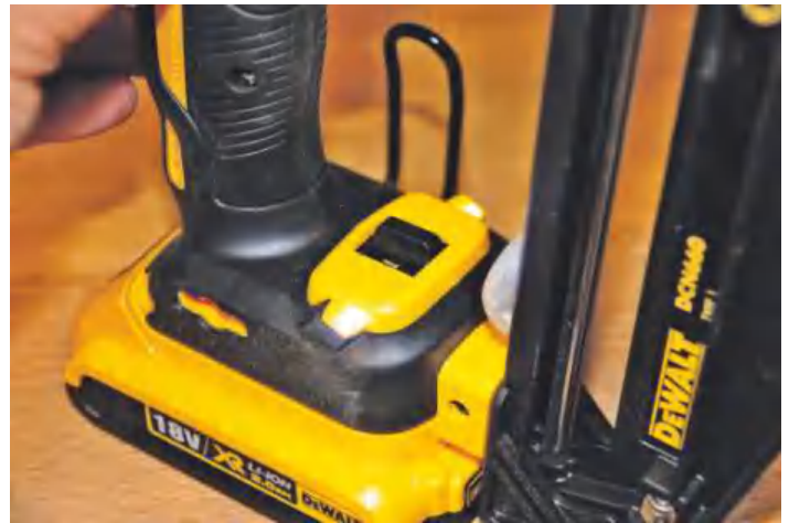
▲ LEDs illuminate the work area and also diagnose basic problems
